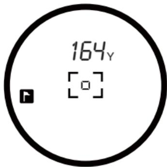
3. Continue looking through the **Eye Piece**, aim the **Zero-In Aiming Square** at your intended target and **PRESS** the **Power Button**. The laser will fire and the **Laser Indicator Box** will appear around the **Zero-In Aiming Square**. The measurement will be displayed at the top of the LCD display.
