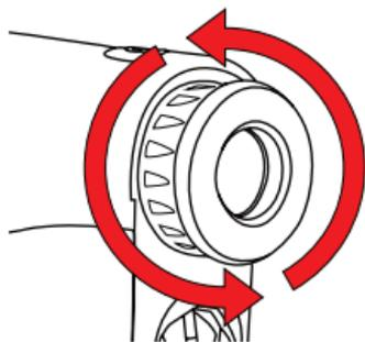
2. To focus/increase clarity, use the **Diopter Adjustment** by turning the **Eye Piece**.
